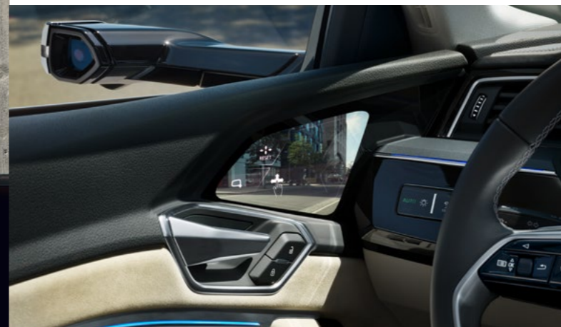
Virtual exterior mirrors. Standard feature for e-tron Sportback, optional for e-tron.
